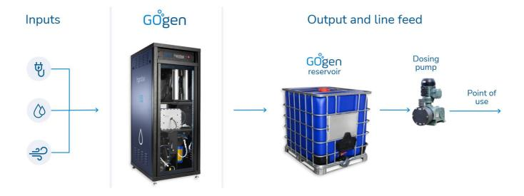
GOgen utilizes only water and electricity as inputs to generate Peroxide UltraPure™ at a safe concentration of up to 1%. The solution is temporarily stored in a buffer tank and dosed into treated water systems at ppm-level concentrations. The buffer tank is automatically refilled based on actual system demand, and remote monitoring of output concentration and key parameters enables process control and preventive maintenance without on-site presence.
