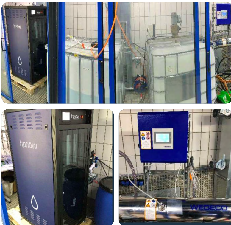
Figure 1: Top: Complete test setup. Lower left: GOgen® H 2 O 2 generator from HPNow. Lower right: Spektron 6 UV-reactor from Xylem
